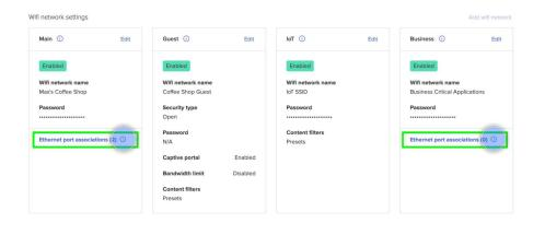
Identify the port to which your device is connected, select the network (SSID) to which you want the device associated, and save your changes. Your hardwired device is now on the same VLAN as the devices that are connected wirelessly on the same SSID.
